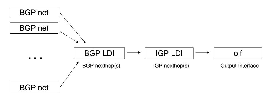
Pointer Indirection between BGP and IGP entries allow for immediate leveraging of the IGP convergence
