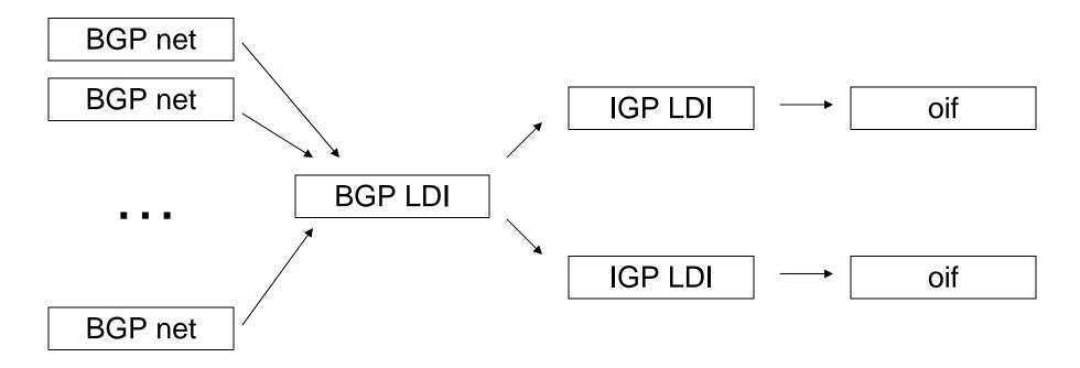
Pointer Indirection between BGP and IGP entries allow for immediate update of the multipath BGP LDI at IGP convergence
