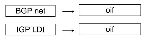
Control Plane flattens the recursion such that any BGP FIB entry has its own local oif information
