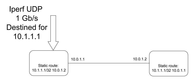
Use the –T option to Iperf to control the number of times the traffic loops Can also use firewall filters to discard a certain TTL range. Other filters may be prudent as well.
