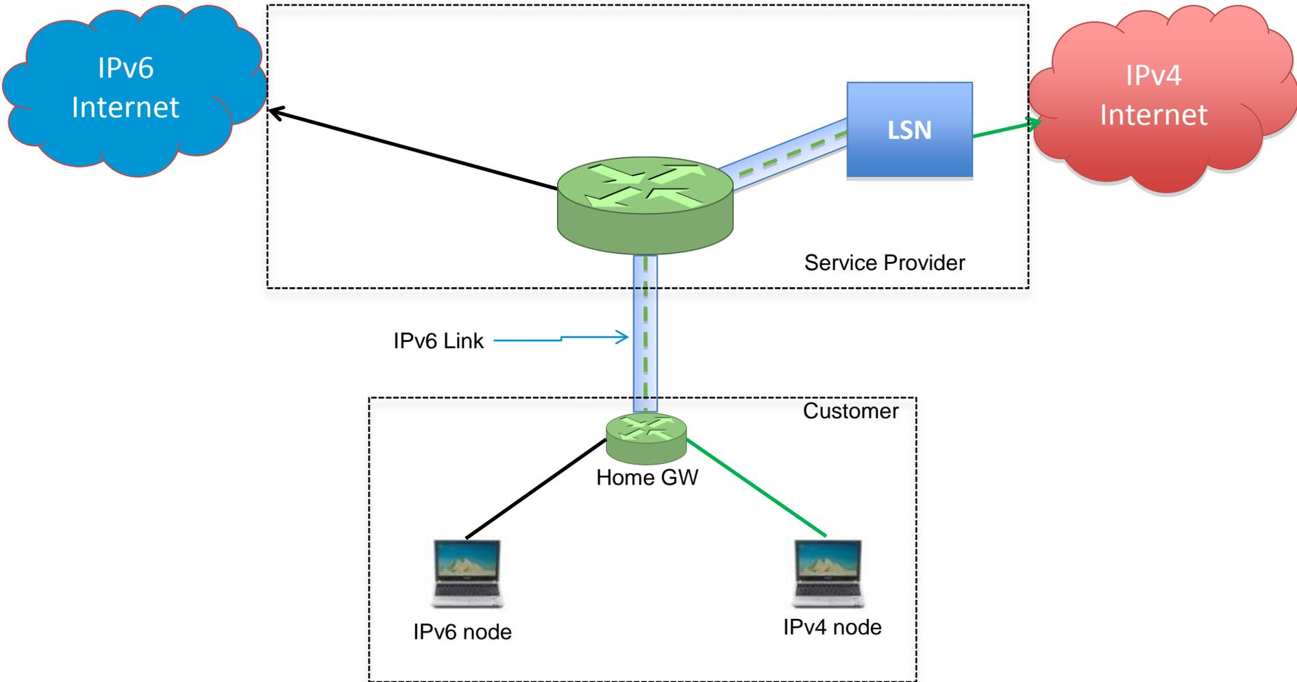
IPv6 packets are routed normally , while IPv4 packets are encapsulated in IPv6 and routed to the LSN
