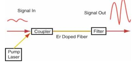
of light in the C-band spectrum, amplifying the signal.
