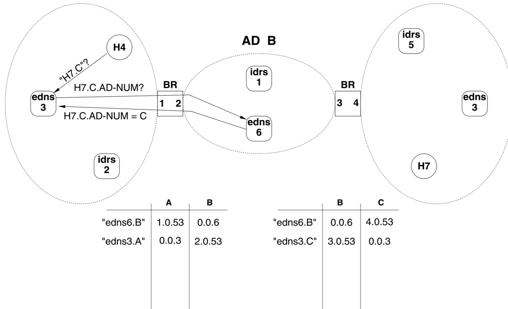
Host H4.A requests IP number for host H7.C. Request percolates through DNS in A and eventually ends up at A's EDNS (**edns3**). First step for EDNS is to find out which AD host H7.C lives in.
