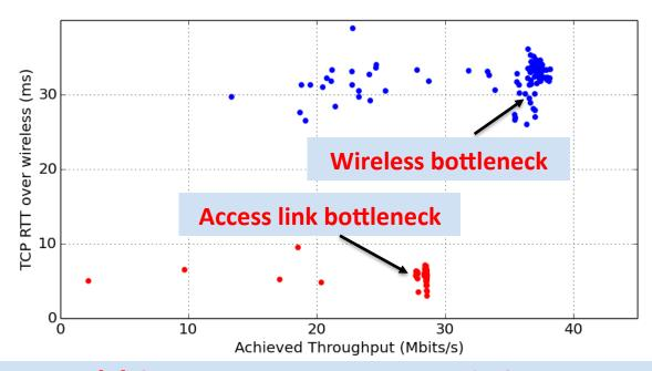
LAN RTT (τ) between gateway and client increases significantly if the wireless is the bottleneck
