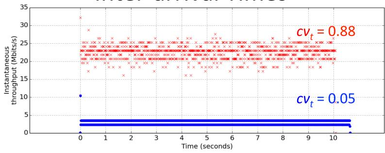
Packets *after* bottleneck have low coefficient of variation of inter-arrival time (cv<sub>+</sub>)
