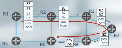
Can shorten label stack by 1 using a node label to get to R7 (and 2 more labels to get to R5).
