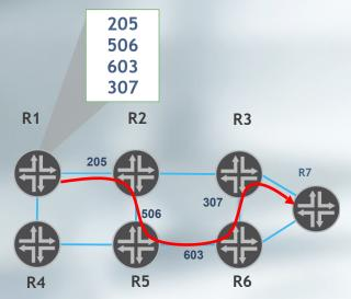
Ingress Router uses a stack of labels to describe a path. The label stack is the ERO.
