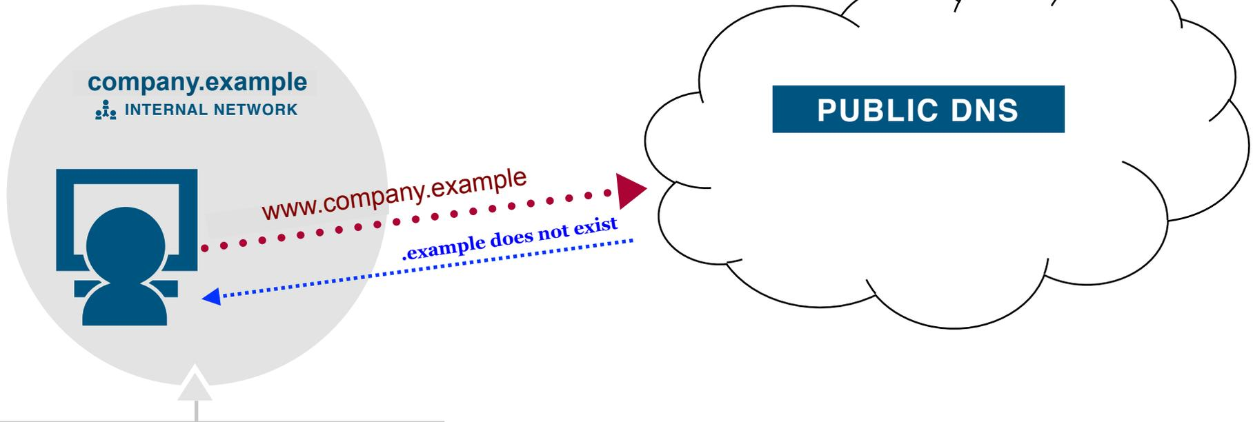
Private network configured in such a way that could “leak” the request to the public Domain Name System, when using a name in a private network that *does not exist* in the public DNS
