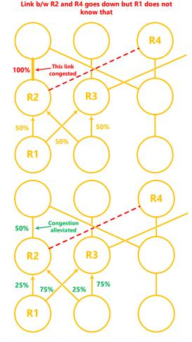
Controller installs path with different ECMP weights
